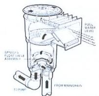
Inside the skimmer body is a round 'well' which contains the 'Skimmer Basket" whose function is the primary 'large object' trap, intended to stop leaves and other large scale debris entering the pump and blocking the impellor.
