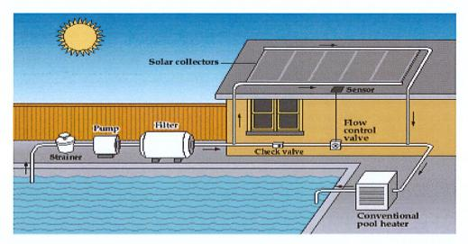
Although the use of solar energy in heating domestic pools is not effective for the entire year, it should work well in the height of summer, but has limited ability to extend the swimming season. They are most effective in mid-summer.
