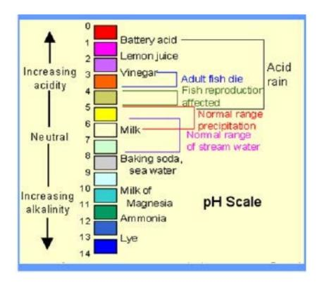
The measure of pH is from 1 (ACID) to 14 (ALKALINE) and keeping within recommended guidelines (7.6) is the most important requirement in keeping your swimming pool water clear and healthy!
